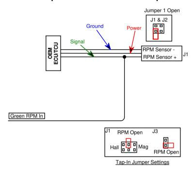
**Note** that Mercury2 or Orion2 ECU's have a green RPM Output on the P2 conectors. This can be tied to the TCU RPM Input directly. Ensure that both ECU and TCU share the same earth point. TCU Input pulses must be the same as RPM output pulses of the ECU.
